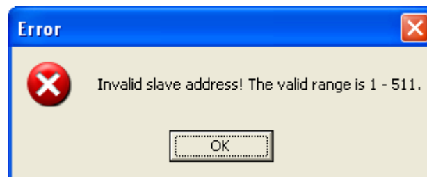
Figure 40: Error Message Box at invalid Slave Address Error
