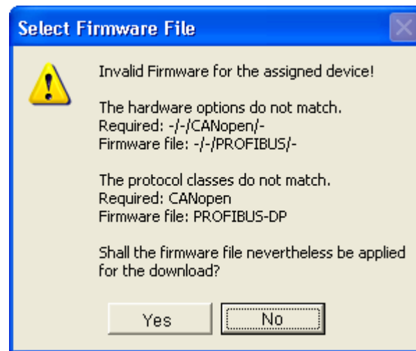
Figure 19: Request Select Firmware File - Example Invalid Firmware
